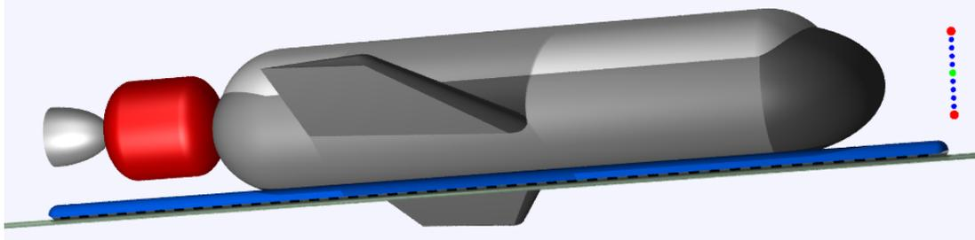
**Figure 11.** A typical 5 ton passenger capsule, with magnet rack, rocket motor for apogee orbit insertion, and wings and a heat shield for accidental reentry. Scale is 1 meter.
