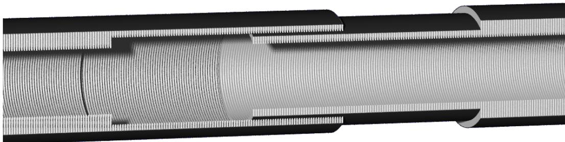
**Figure 7. Joint for a 2 meter rotor segment. The core may consist of laminated iron, or a weave of iron wire. The surface is smooth carbon to minimize sputtering.**
