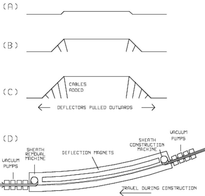
**Figure 6. Deploying the Launch Loop.**
